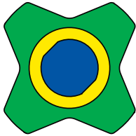
Industrial/Process Water, Cold
