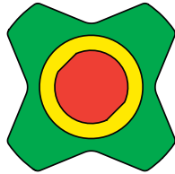
Industrial/Process Water, Hot
